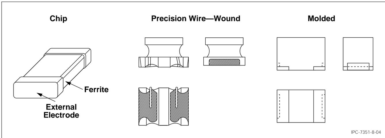
Figure 8-4 Inductor Construction
