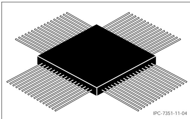
**Figure 11-4 CQFP Construction**
