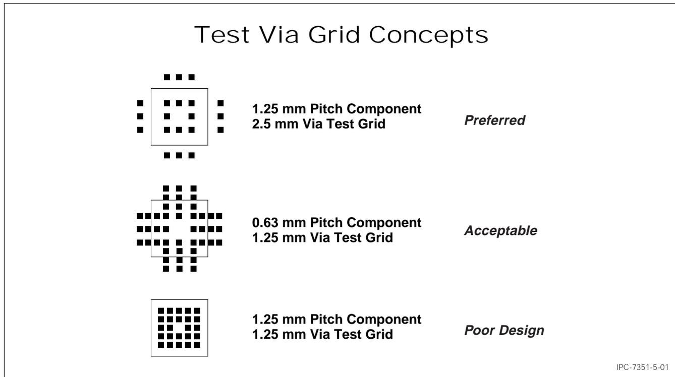
**Figure 5-1 Test Via Grid Concepts**
