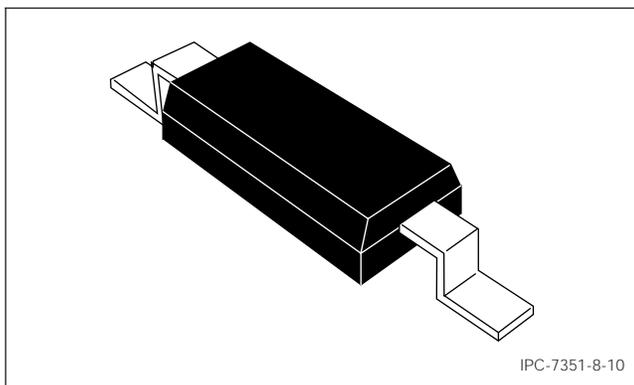
Figure 8-10 SOD 123 Construction
