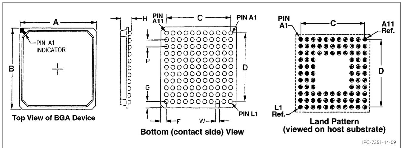
**Figure 14-9 Device Orientation and Contact A1 Position**
