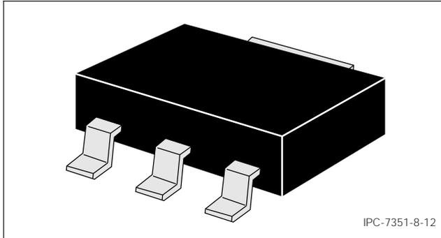
**Figure 8-12 SOT 223 Construction**
