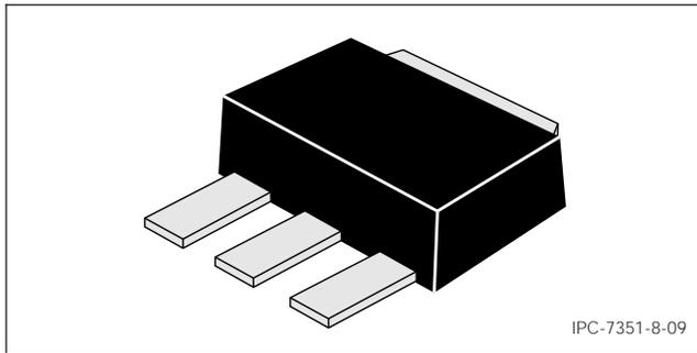
Figure 8-9 SOT 89 Construction
