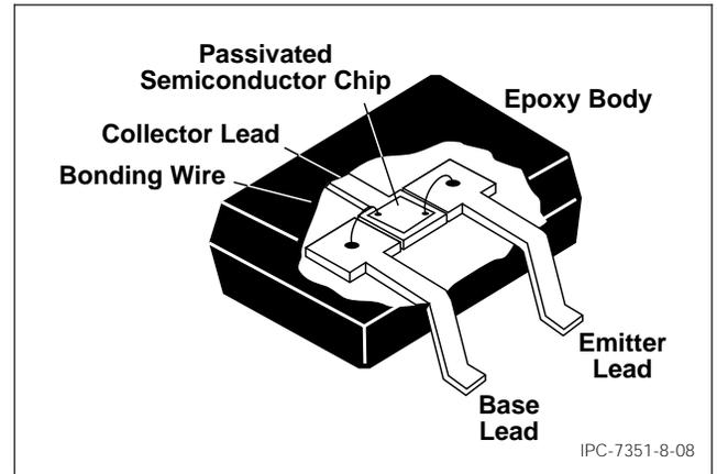
**Figure 8-8 SOT 23 Construction**
