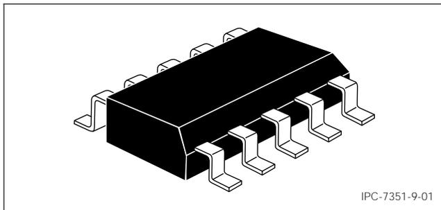
Figure 9-1 SOIC Construction
