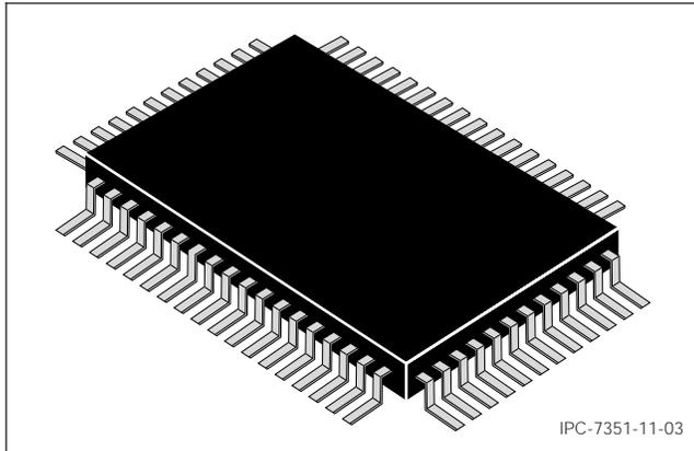
**Figure 11-3 QFPR Construction**
