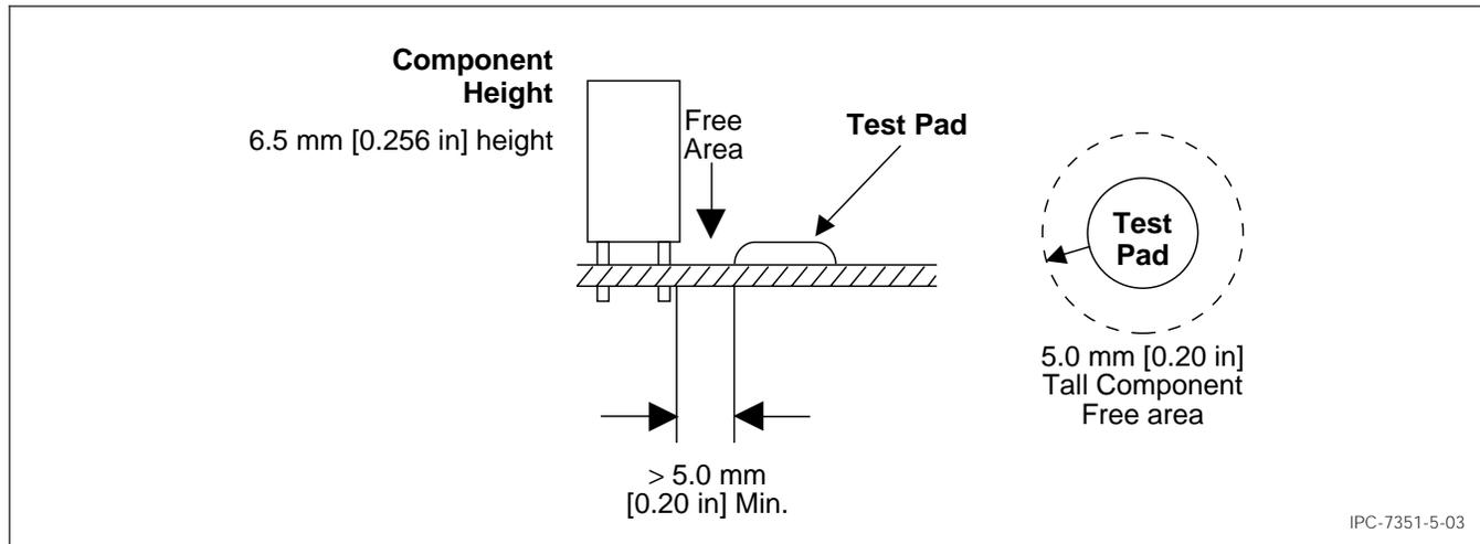
Figure 5-3 Test Probe Feature Distance from Component
