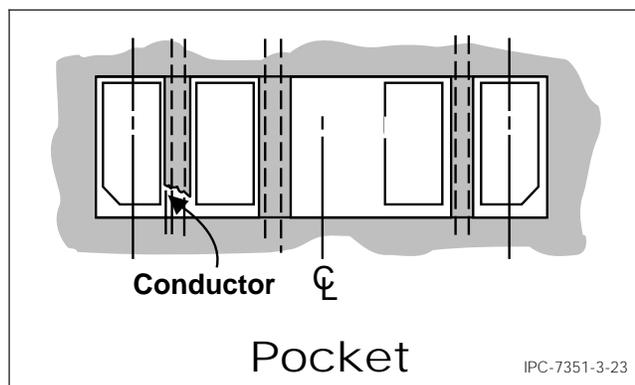
Figure 3-23 Pocket Solder Mask Window
