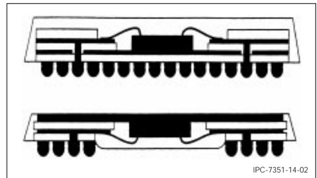
Figure 14-2 Example of Plastic BGA Package Configurations
