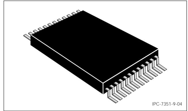
**Figure 9-4 TSSOP Construction**
