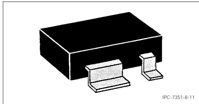
Figure 8-11 SOT143 Construction
