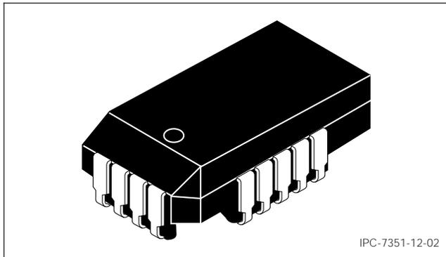
Figure 12-2 PLCCR Construction
