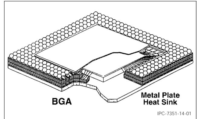
Figure 14-1 Ball Grid Array (BGA) IC Package Example
