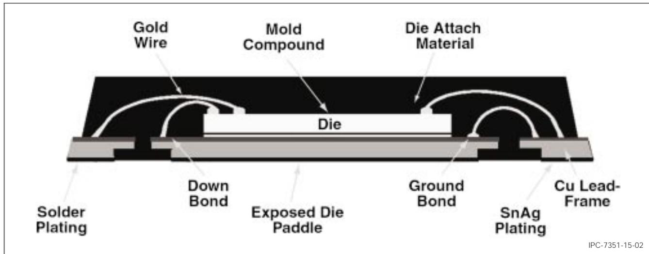
Figure 15-2 Quad Flat No-Lead (QFN) Construction (Cross-Sectional View)
