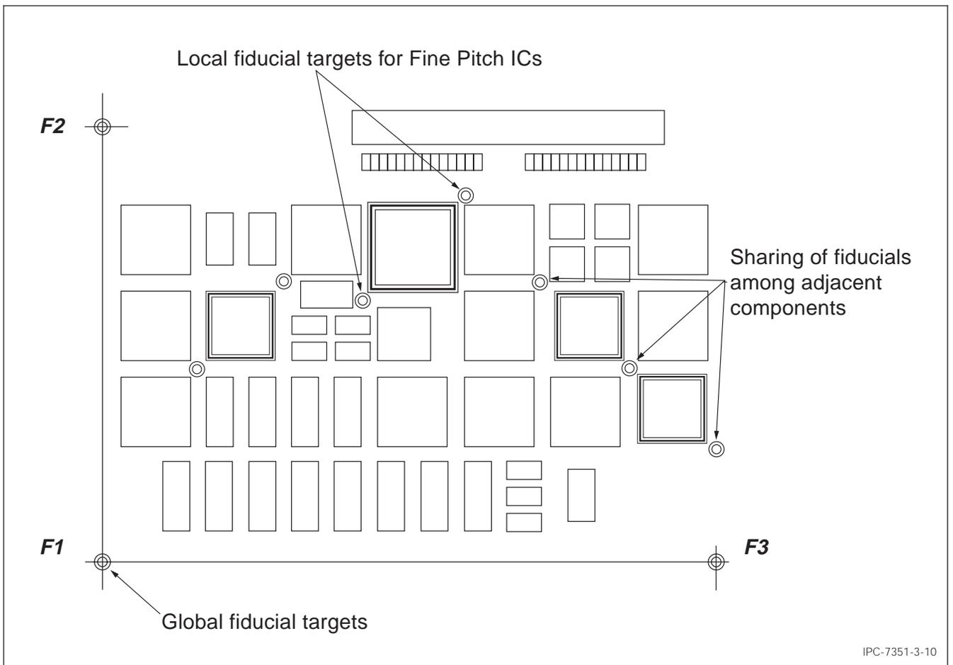
Figure 3-10 Fiducial Locations on a Printed Board
