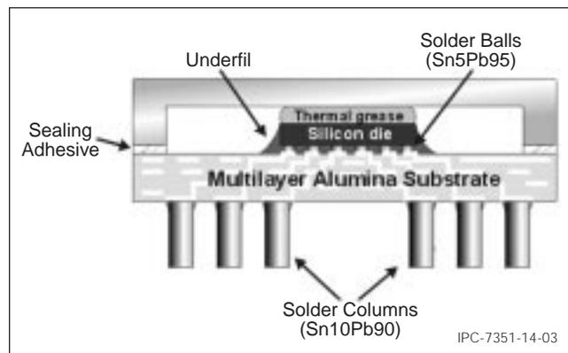
**Figure 14-3 Ceramic Column Grid Array (CGA) Package
