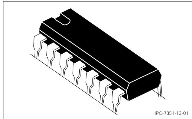
Figure 13-1 DIP Construction
