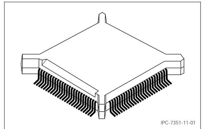
Figure 11-1 BQFP Construction
