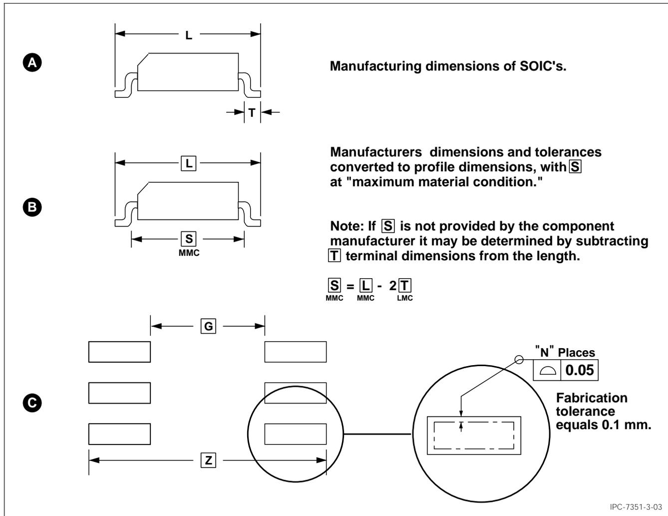
Figure 3-3 Profile Dimensioning of Gull-Wing Leaded SOIC
