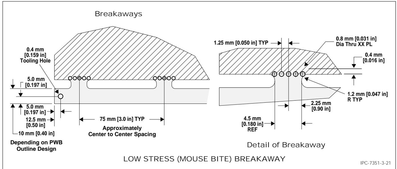
Figure 3-21 Breakaway (Routed Pattern) with Routed Slots
